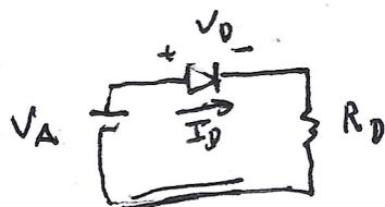
$$V_A = V_D + I_D R_D \Rightarrow V_A = V_D + I_0 (e^{qV_D/kT} - 1) R_D$$
